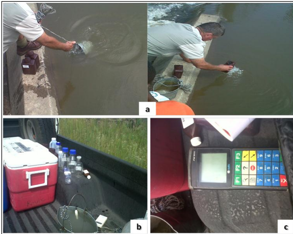
Figure 37: Grab method as performed by Rand Water technician (a) and bottles (b) and instrument (c) used during the water sampling campaign [Ambani, 2012]
